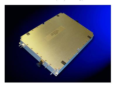
Standard housing size is approximately 4.75 X 7.75 X 1.00 inches not including the mounting flange. SMA female connectors are standard in the RF input and output ports. DC, command/control signals are accessible via DC feed through capacitors.
