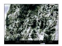
Picture taken at 1,000x magnification using a SEM to demonstrate the fibrous nature of the FlexiCap<sup>TM</sup> termination that absorbs increased levels of mechanical stress.
