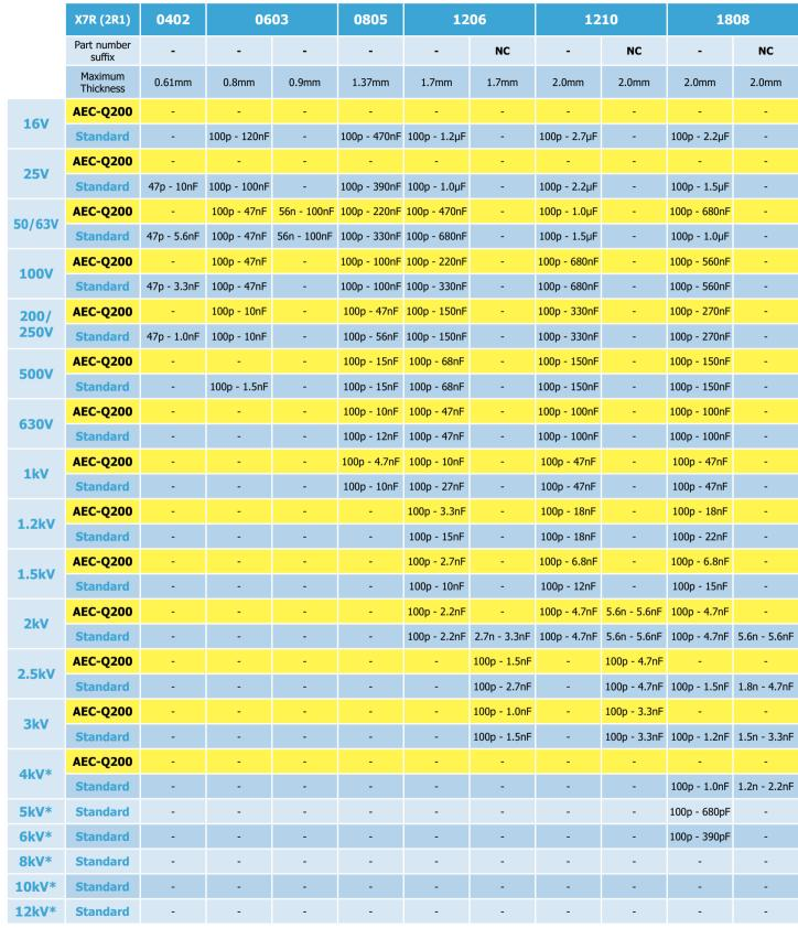
Notes: 1) \*Parts rated 4kV and above may require conformal coating post soldering.
