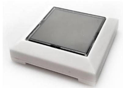
EMSIU provides an integrated NFC interface that can be used for device configuration and device commissioning and an LRN button that can be used for simple commissioning tasks.
