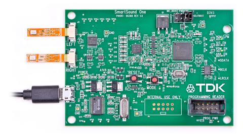
SmartSound One features an EEPROM to load the factory default DSP program on power up, making it a plug-and-play solution. There are two parallel signal processing paths for analog and digital microphones which the user can select using the 'mode' button which is routed through the DSP and the on-board USB audio codec to send audio data packets over USB.
