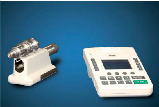
Upside down measurement with vee-block Automatic zero setting of the BFW 250
