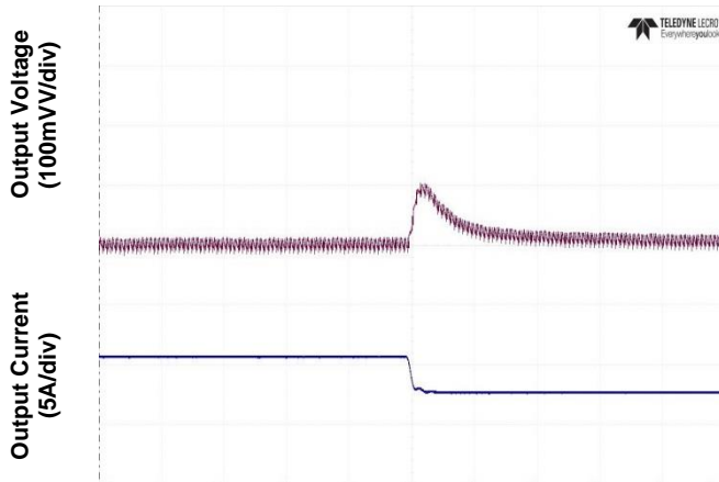
Figure 7. Transient Load Response at V_o=3.3V ( V_{in}=12V ; I_o=6A \rightarrow 3A @ 0.5A/\mu s ; C_{o,ex}=220\mu F )
