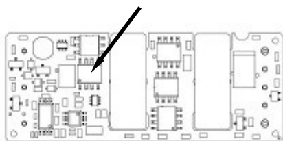
Figure 22. Temperature Monitoring Location
