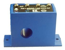
AG Series products with solid state outputs combine the benefits of NK Technologies' ground fault sensing technology with the reliability and longevity of solid state contacts. Solid state technology provides unlimited switch operating life, superior resistance to shock and vibration, zero off-state leakage, high switching speeds and high input-output isolation, all of which make these units an ideal choice for standard and harsh environments alike.
