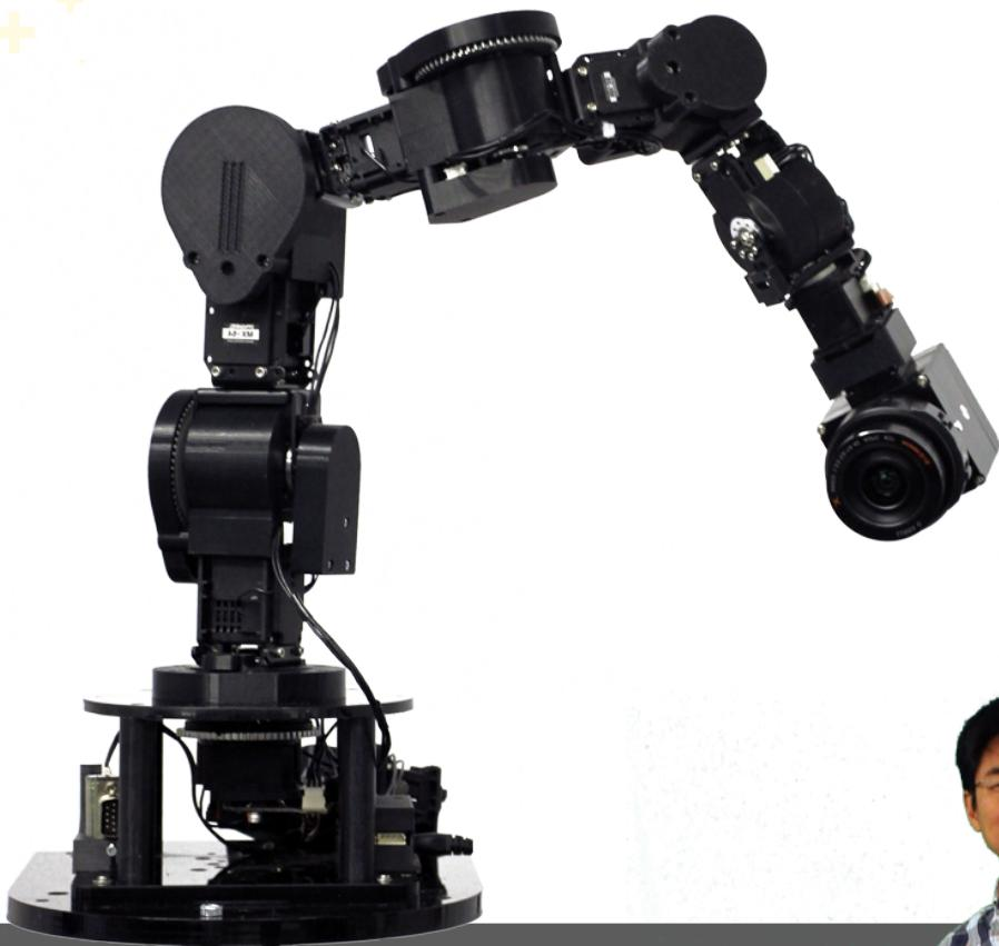
Humanoid robot arms offer significant advantages. With many degrees of freedom, they are able to reach around obstacles and through passageways, reconfigure for strength, and manipulate objects with dexterous fluid motion.
