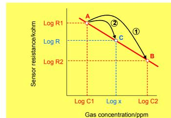
Plot A and B: Calibration point Plot C: measuring point
