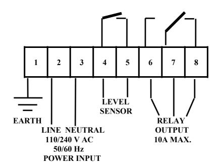
Terminal 1 should be connected to earth
