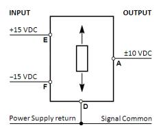
A through F: Connector pin assignments
