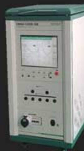
• 10kV 5kA Surge Test
